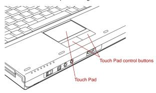
Figure 4-1 Touch Pad and Touch Pad control buttons
